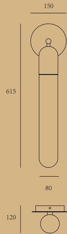
ITEM No.: MB1116-1 FINISH: Matte copper + white glass MATERIALI: Copper + aluminum + glass POWER SQRGE: AC 220-240V WATTAGE: GU10 LED 7W 2700K
