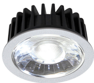
DISC LED insert MR16, 6 W, with lens optics, 350 mA, CRI > 80
