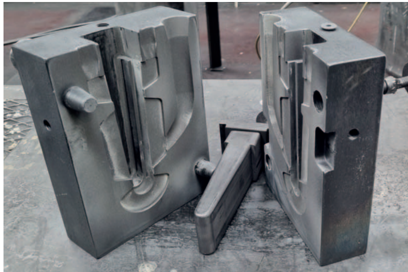
Jig used to make the brackets connecting the vertical elements fixed to the wall and the shelves. The brackets are made of cast aluminium.
