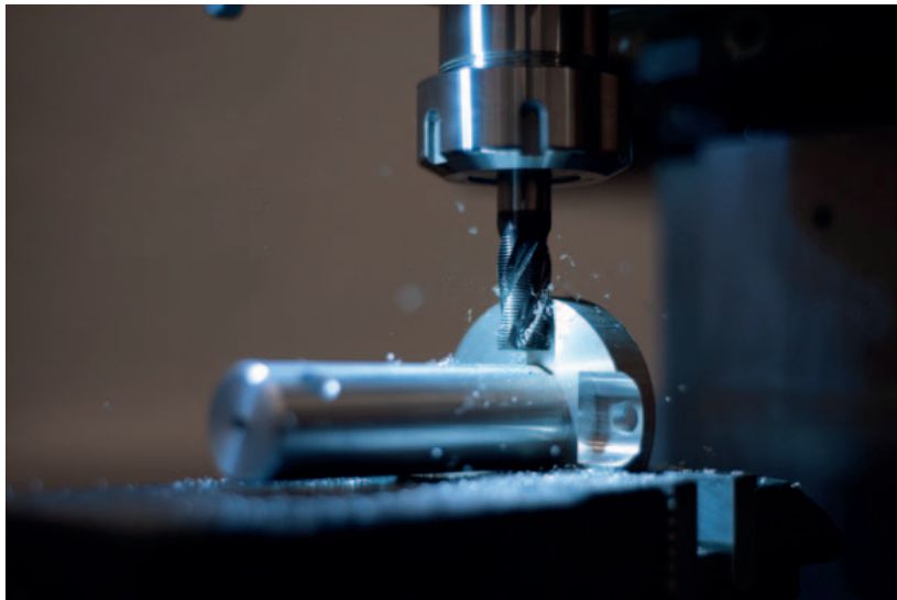
CNC machining of the aluminium elements that make up hub.
