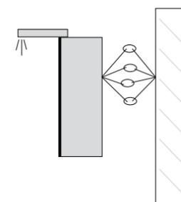
Four-wire mirror cabinet cable is connected to four-wire wall cable.
