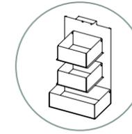
Tiered holder, side, including 3 boxes (2 boxes: 70 x 35 x 70 mm, 1 box: 110 x 35 x 70 mm), for suspending at the rear or on the side under the shelf, white aluminium finish
