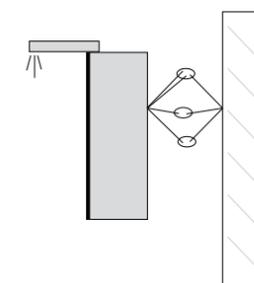
Four-wire mirror cabinet cable is connected to three-wire wall cable. Two lines must be laid to one wall connection.
