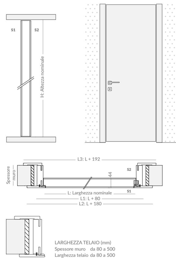
Coplanarity of the door with strip covers on the push side with full-height opening. In combination with Ghost freewall, Planya freewall allows all doors in the same room to be coplanar. This system is also available in all lacquered models, standard finishes and on request.
