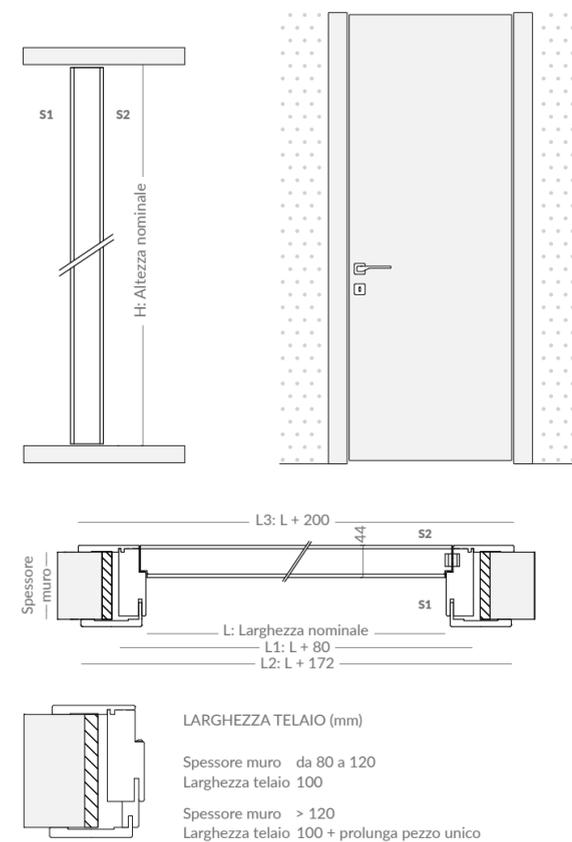
Coplanarity of the door with strip covers on the pull side with full-height opening. In combination with Planya freewall, Ghost freewall allows all doors in the same room to be coplanar. This system is also available in all lacquered models, standard finishes and on request.
