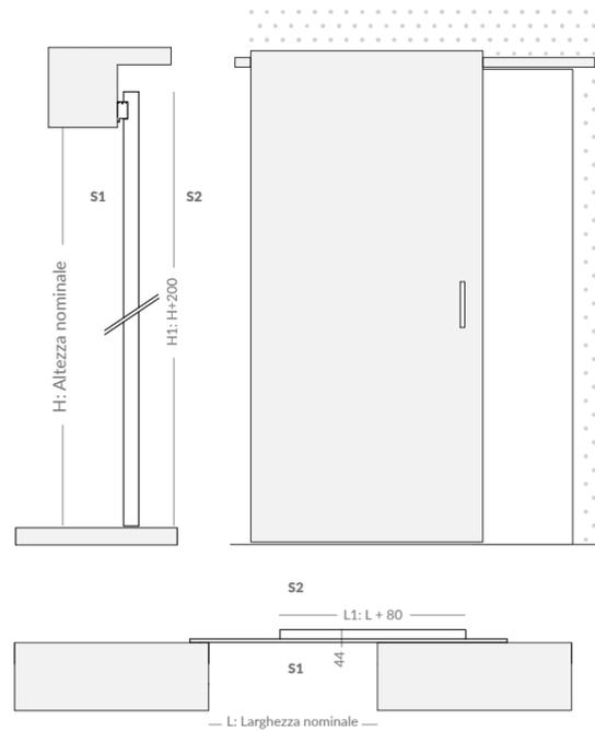
Single- or double-panel sliding door with visible slide. This system is also available in all lacquered models, standard finishes and on request.
