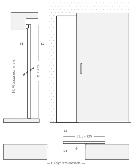
Single-panel sliding door with retractable slide. This system is also available in all lacquered models, standard finishes and on request.
