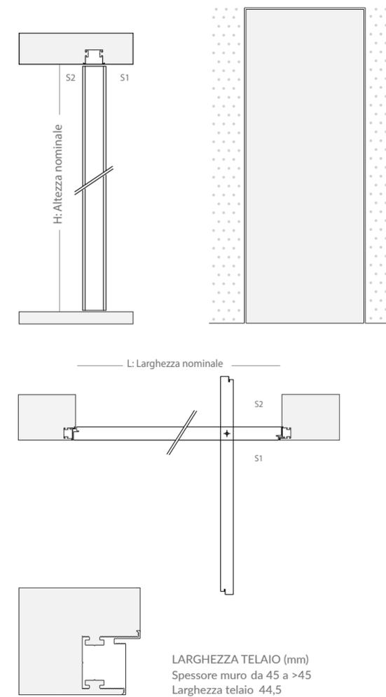
Flush-wall pivot door on pull side with full-height opening. In combination with Level Flag Push, Level Flag Pull allows all doors in the same room to be flush to the wall. This system is also available in all lacquered models, standard finishes and on request.
