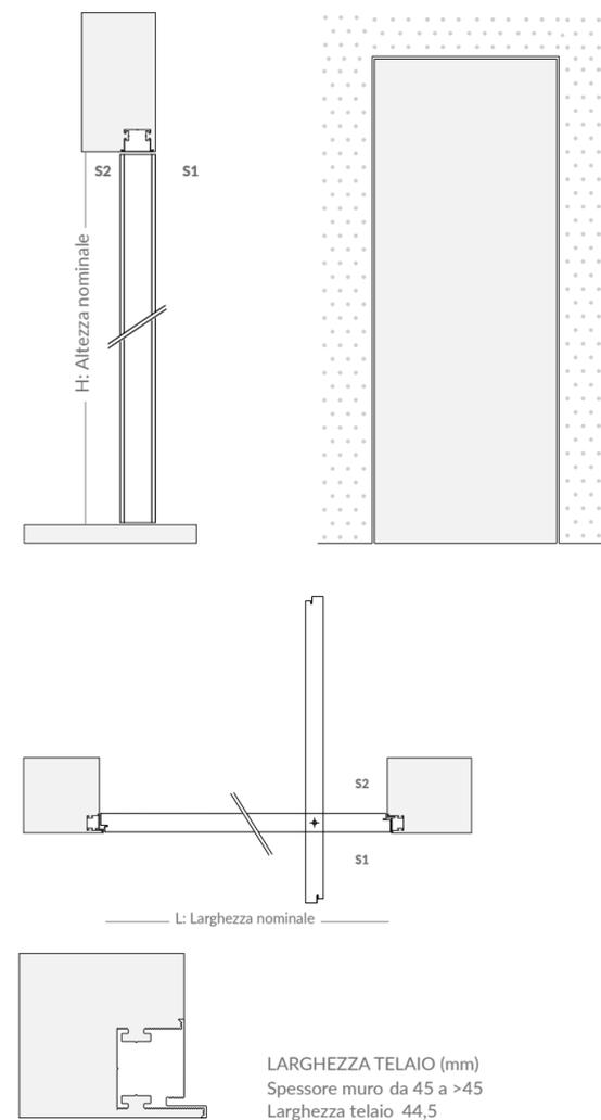
Flush-wall pivot door on push side. In combination with Level Flag Pull, Level Flag Push allows all doors in the same room to be flush to the wall. This system is also available in all lacquered models, standard finishes and on request
