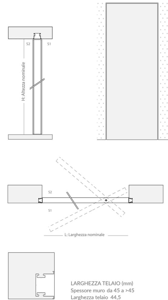
Free pivot door with full-height opening. This system is also available in all lacquered models, standard finishes and on request.
