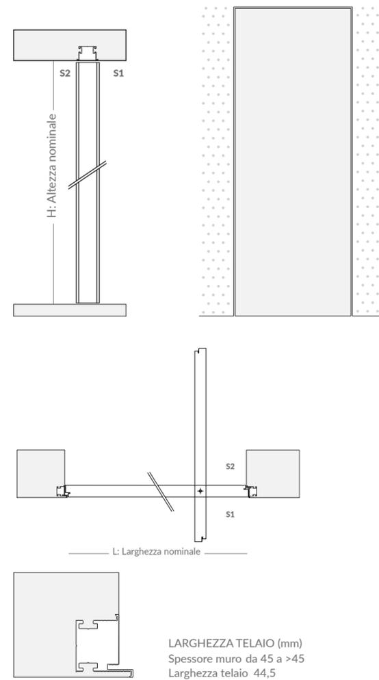
Flush-wall pivot door on push side with full-height opening. In combination with Level Flag Pull, Level Flag Push allows all doors in the same room to be flush to the wall. This system is also available in all lacquered models, standard finishes and on request.
