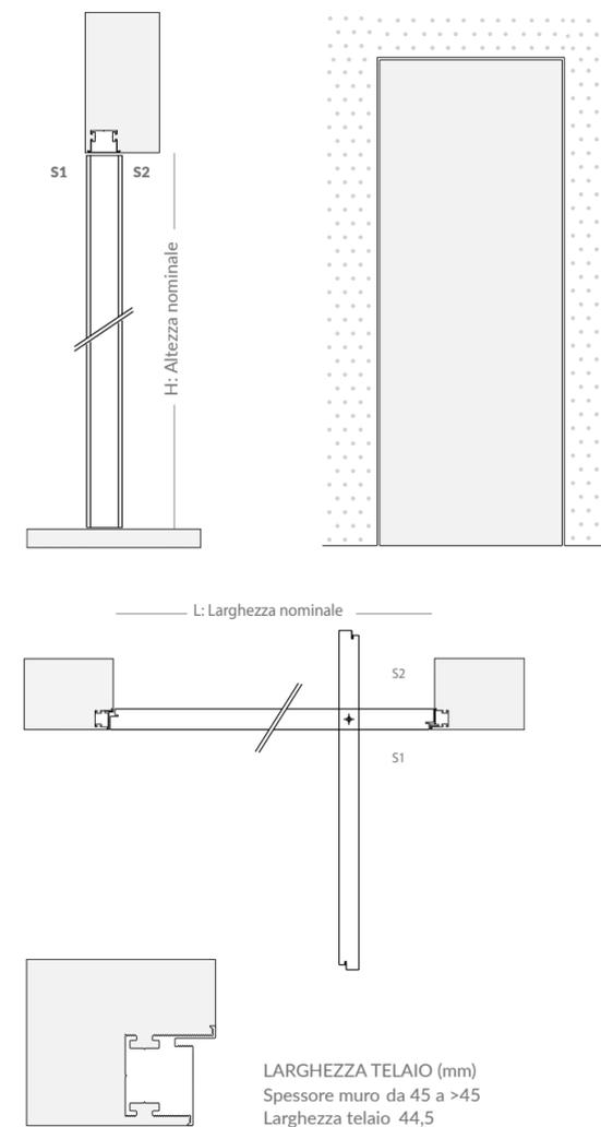
Flush-wall pivot door on pull side. In combination with Level Flag Push, Level Flag Pull allows all doors in the same room to be flush to the wall. This system is also available in all lacquered models, standard finishes and on request.
