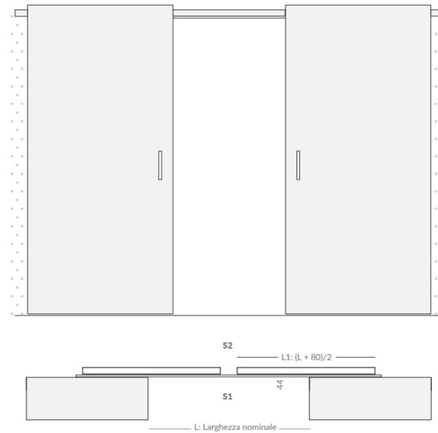
Single- or double-panel sliding door with full-height opening and visible slide. This system is also available in all lacquered models, standard finishes and on request.
