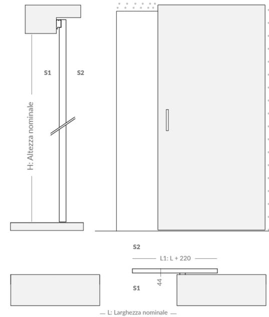
Single-panel sliding door with full-height opening and retractable slide. This system is also available in all lacquered models, standard finishes and on request.
