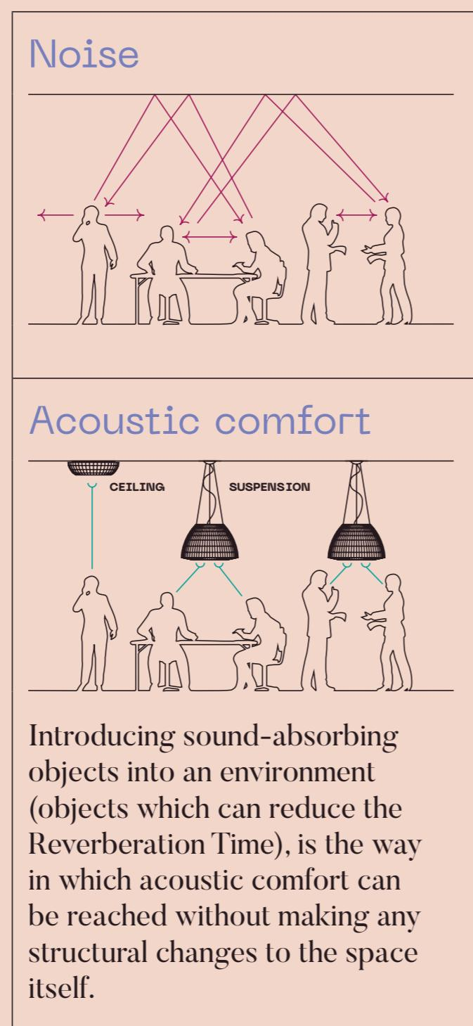
Introducing sound-absorbing objects into an environment (objects which can reduce the Reverberation Time), is the way in which acoustic comfort can be reached without making any structural changes to the space itself.
