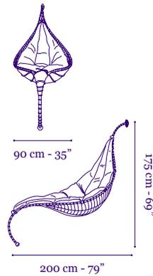
The unique design, supported on one leg, allows the user to rock themselves once reclined. Suitable for indoor or outdoor use where sheltered, the Satala is made of galvanised metal painted in a bronze shade with a range of fabric colors or customer's own material used for the removable down-filled cushion.
