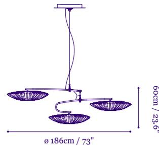
Cable length is not included within the 60cm / 23.6" height measurements.
