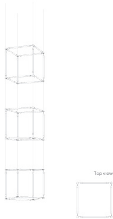
CGV06 Dimensions: 1000 × 1000 × 5000 mm Number of crystal components: 36 pcs Number of connectors: 24 pcs
