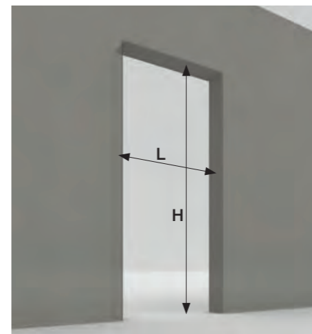
Rilievo misure del vano Wall opening measuring
