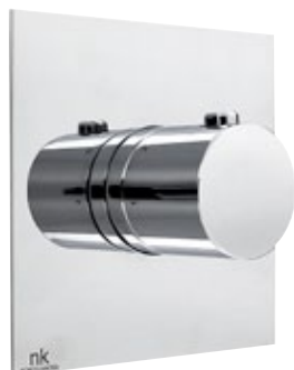
GIRO Termostática encastre con termoelemento de cera incorporado. Conexiones de 3/4". Incluye válvula anti-retorno y stop de seguridad a 38°C. Concealed thermostatic 3/4" with wax thermostatic element. Built in non-return valve, safety stop at 38°C (for a correct use this item needs to be combined with a deckmounted control).
